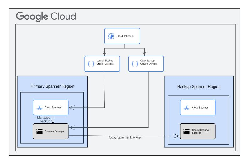
In the case of a failure scenario where the main region becomes unavailable, these backups in the backup region can be used to restore and populate a Spanner database in the backup region.
