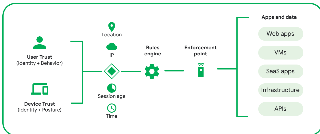
Figure 15: A Zero Trust security model with various device and user signals helping a company determine access
